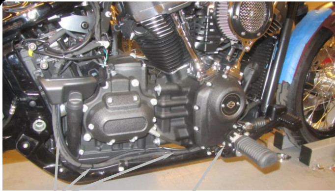
ROUTE FRONT O 2 HARNESS ALONG EXISTING WIRE HARNESS; ZIPTIE HARNESS TO EXISTING HARNESS WITH 4" ZIPTIES
