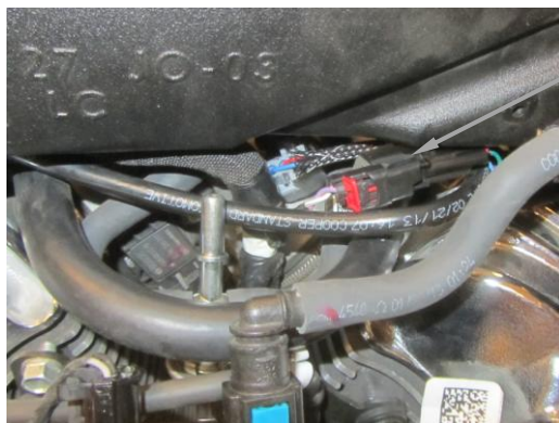
FIGURE 11 (FRONT INJECTOR CONNECTOR INSTALL)
