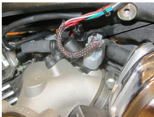
FIGURE 9 (REAR INJECTOR CONNECTOR INSTALL)
