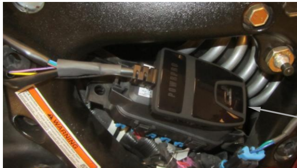
FIGURE 7 (POWRPRO INSTALL LOCATION)
