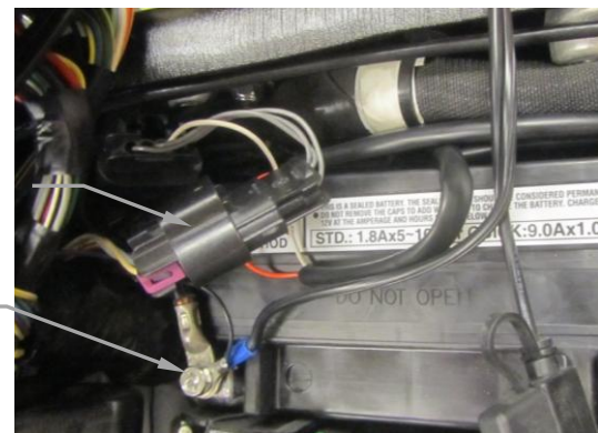
FIGURE 12 (REAR O 2 AND GROUND WIRE CONNECTION)
