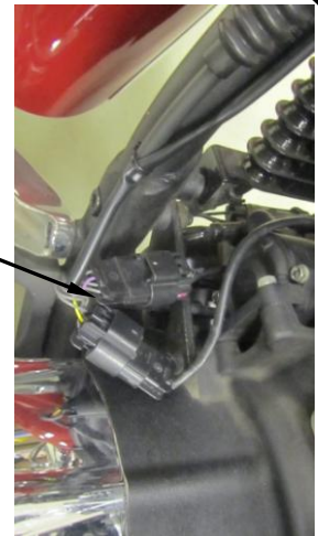
FIGURE 14 (FRONT O 2 CONNECTORS)
