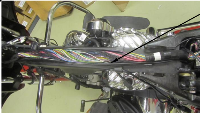
FIGURE 13 (FRONT O 2 HARNESS ROUTING)
